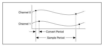
Figure B-1. ai/SampleClock and ai/ConvertClock
